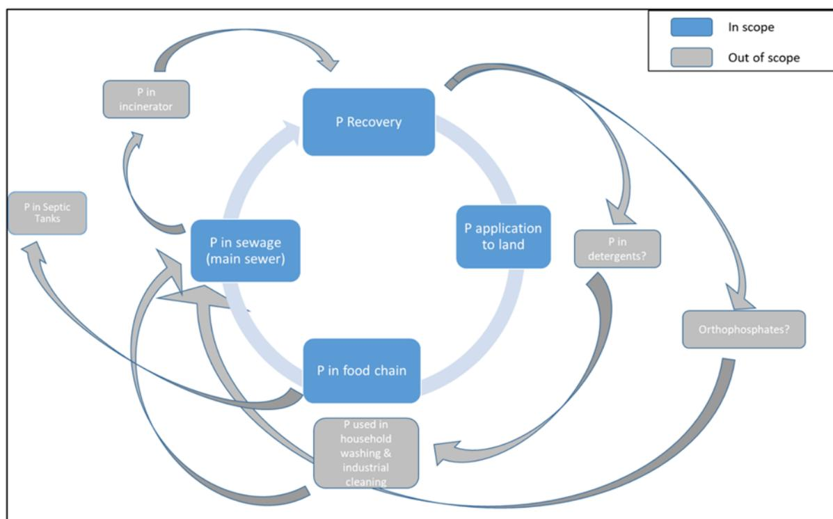
**Figure 6.1.2: The phosphorus recovery cycle**
