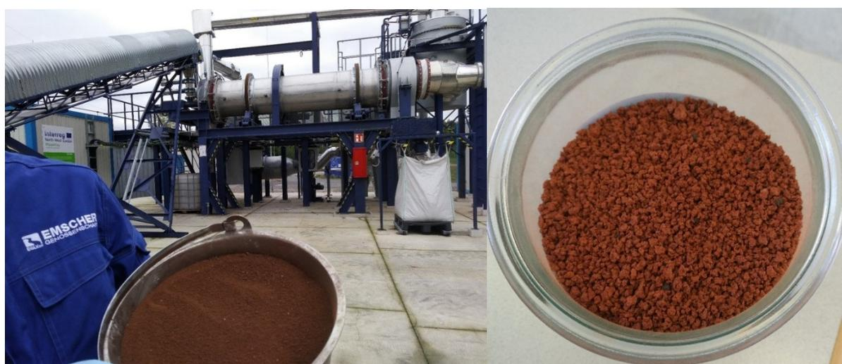
**Figure 3.2.1 a and b: Physical appearance of the ashes coming out of the EuPhoRe® process**
