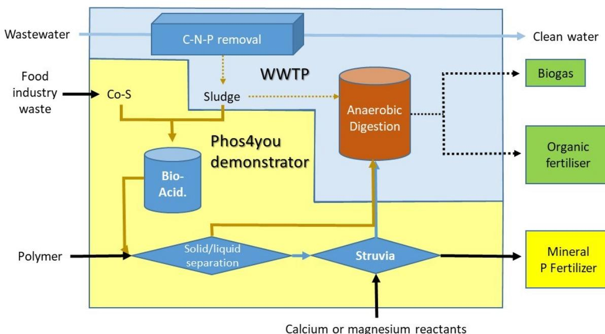
**Figure 3.3.1: Implementation of the bio-acidification process in WWTP**
