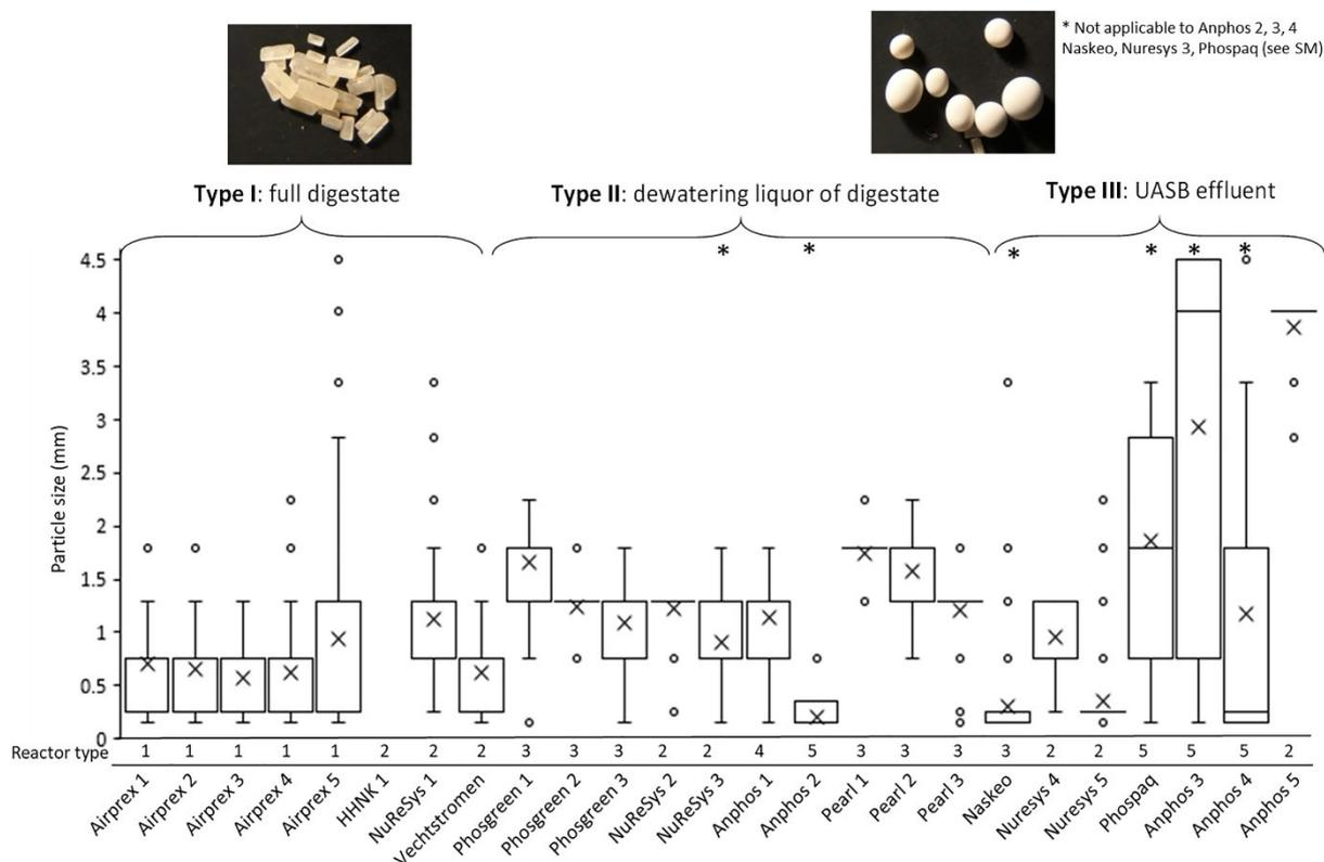
**Figure 4.1.3: Mass fraction distribution per particle size for all analysed struvite samples. Crosses indicate the mean particle size (mm). Numbers indicate the reactor type as follows: 1 Airlift reactor, 2 Continues stirred tank reactor, 3 Fluidized bed reactor, 4 Tank aerated, 5 Tank mixed (Muys et al. 2021).**
