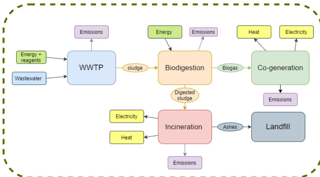
**Figure 3.8.2: System boundaries for the reference case with the avoided burden approach (Chantrain et al. 2021)**
