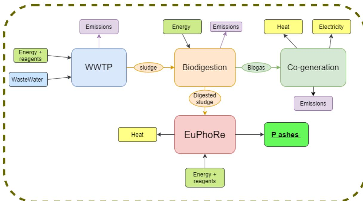
**Figure 3.8.3: System boundaries for the EuPhoRe<sup>®</sup> system with the avoided burden approach (Chantrain et al. 2021)**
