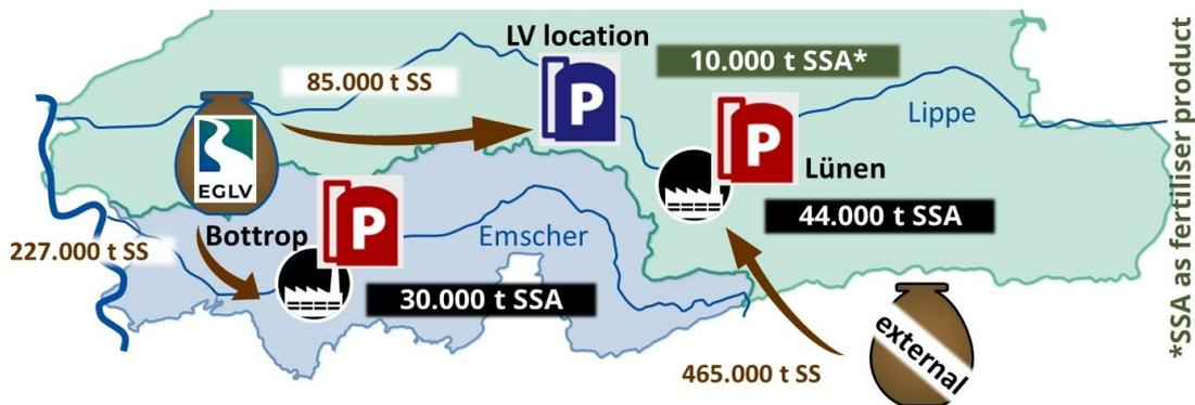
Figure 5.3.6: Schematic illustration of a possible extension of the in-house model implementing both, a wet-chemical recovery and a thermochemical P-recovery (Blöhse et al. 2021)
