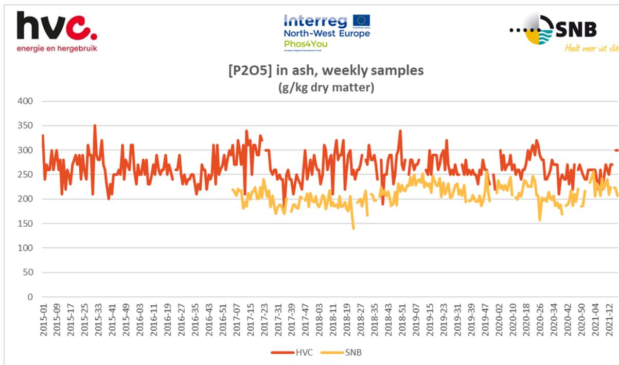
Figure 5.2.2: P<sub>2</sub>O<sub>5</sub> content in sewage sludge ashes of HVC and SNB (Ruijter et al. 2021)
