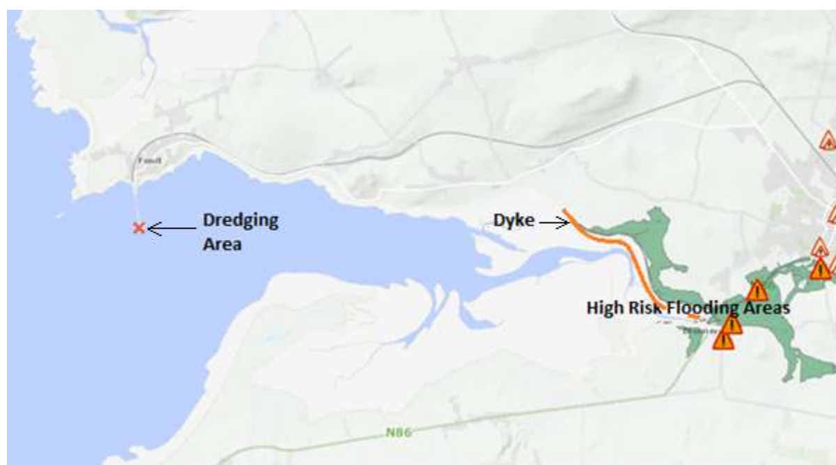
Figure 2-6: Proposed dyke location and areas of high flood risk in Tralee Bay
