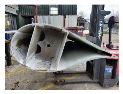
Figure 3. Cross-section of the LM 13.4 blade at maximum chord.
