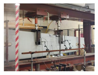
Figure 5. Structural testing of the LM 13.4 wind blade in the MTU structures laboratory.
